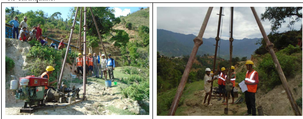
Pictures: Extracting the underground sample soil for testing
